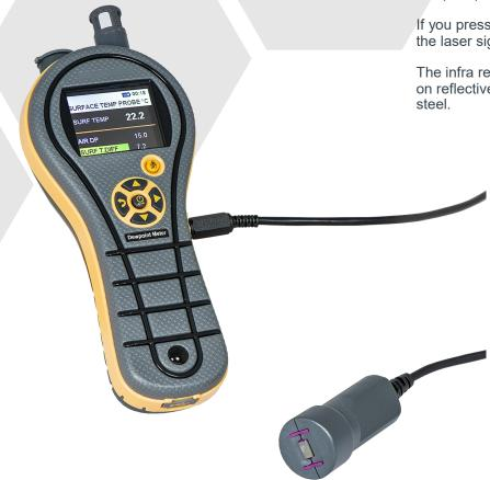
When the surface Probe is placed on the steel substrate the Surface Temperature Difference measurement must be over 3°C to ensure that there is no moisture on the steel before painting.
